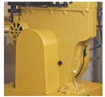
A huge iron casting provides a solid foundation that keeps the PWBS-14 rigid and vibration free.
